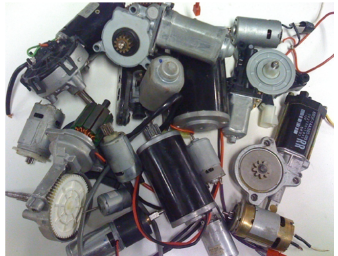
Figure 1: A number of sizes of Permanent Magnet DC motors.
